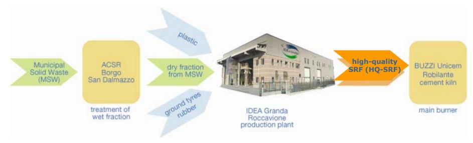
The cement kiln currently substitutes approx. 40% of coal-petcoke consumption by using HQ-SRF in its main burners.
